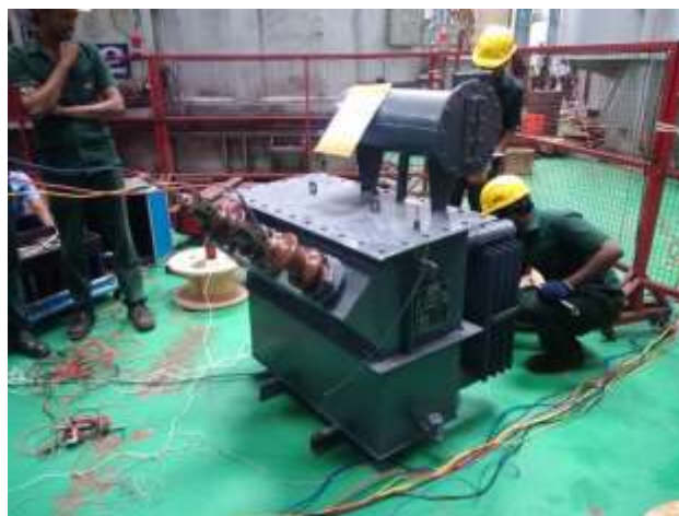
Figure 14. Setting up connections for enhanced capacity testing at NABL
