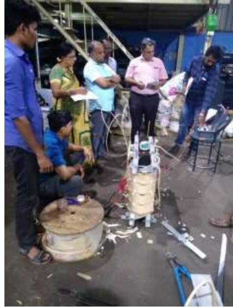
Figure 10. Final repaired DT ready for post repair testing
