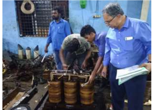
Figure 2. Dismantling and inspection of transformer
