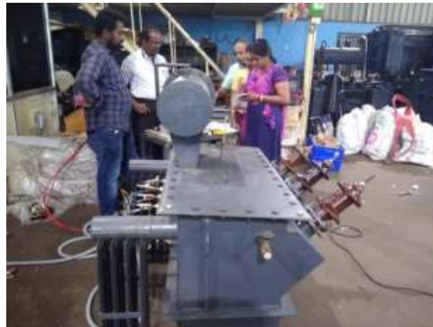
Figure 12. Post Repair testing and recording measurements
