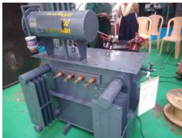
Figure 18. Final repaired DT ready for reconnecting in the network
